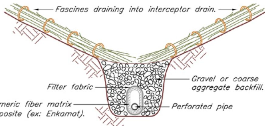
CROSS-SECTION OF SUBSURFACE
