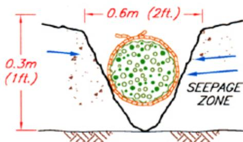
Excavate a shallow trench or utilize existing "seepage gully" (small <2ft.<sup>2</sup>).
