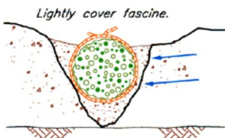
Place bundle of cuttings (fascine) in the trench and lightly backfill with native material.
