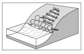
repairing elongated voids in a slope, such as gullies. Gully treatment must include correcting or eliminating the initial cause of the gully as well as the gully itself. Accordingly, consideration should be given to diverting excessive or concentrated runoff away from the gully head area. Gullies are likely to have side gullies that require treatment; however, priority should be given to the main channel.
